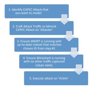
Figure 2. Process used to capture the attack traffic
